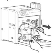
${\it 3}$  Press and hold down the cassette button, and remove the retransfer film cassette (on the left) to remove the retransfer film
