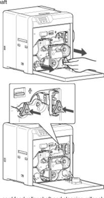
Turn the card feed roller shaft and cleaning roller shaft in the clockwise direction, while checking the position of the card
