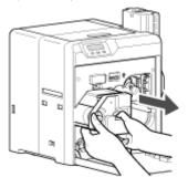
4 Apply alcohol to a cotton swab (large), and use it to wipe the four bobbin holders
