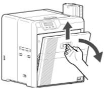
2 Press and hold down the cassette button, and remove the ink ribbon cassette (on the right) to remove the ink ribbon
