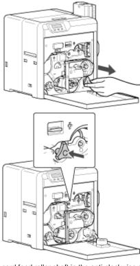
4 Turn the card feed roller shaft in the anti-clockwise direction, while checking the position of the card
