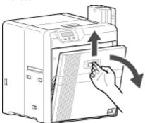
2 Press and hold down the cassette button, and pull out the retransfer film cassette (on the left) to remove the retransfer film
