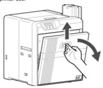
2 Press and hold down the cassette button, and pull out the ink ribbon cassette (on the right) to remove the ink ribbon
