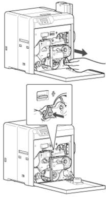
Turn the card feed roller shaft in the anti-clockwise direction, while checking the position of the card
