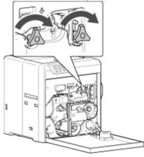
Remove the card after it is discharged from the card load slot. (For single-sided printers, the card is discharged from the NG card outlet.)
