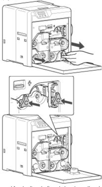
4 Turn the card feed roller shaft and cleaning roller shaft in the clockwise direction, while checking the position of the card
