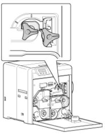
• If the card protrudes from the card turn over unit, turn the cleaning roller shaft to move the card into the unit.
