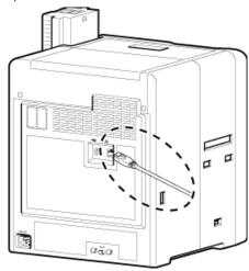
${\it 3}$  Plug the LAN cable into the connection terminal of the hub that is installed on the network that the computer is connected to
