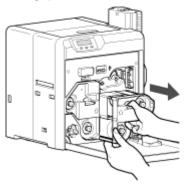
3 Cut away the broken portion, and attach the unused portion at the supply side to the other end at the take-up side using an adhesive tape, while making sure that the joint surface is even
